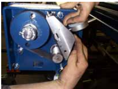
pic 17: Put the measuring device on the V-belt
