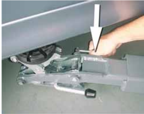
Pic 3: Press the rear lever to unlock the pads.
