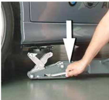
Pic 2: Press the lever to position the pads under the pick-up points.
