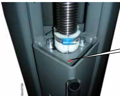
pic 18: the carrying-nut wear pin marked with red safety colour
