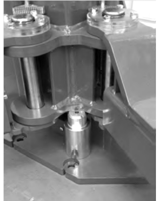
Diagram 5 – Using Pad Adaptors for Gauging Balance Cable Adjustment
