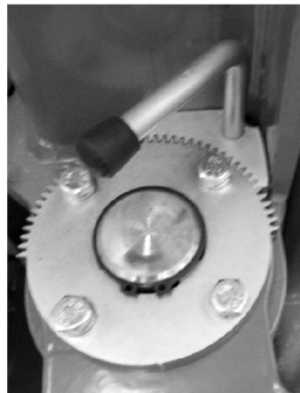
Diagram 4B – Arm Lock fully engaged.
