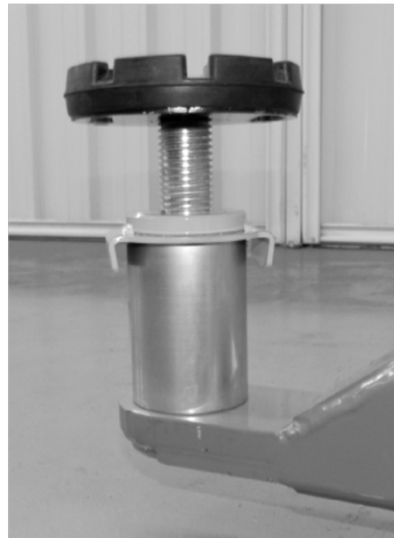
Diagram 2B - Pick-up pad on extension adaptor and adjusted up to its maximum height.
