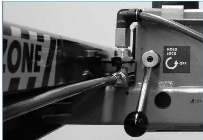
Photos of Coiled Hose (#11) fitted over wire rope assembly between bulkhead and jacking beam.
