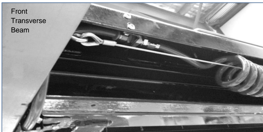
Photo of Bulkhead components attached, under front of Left Hand Platform lip.
