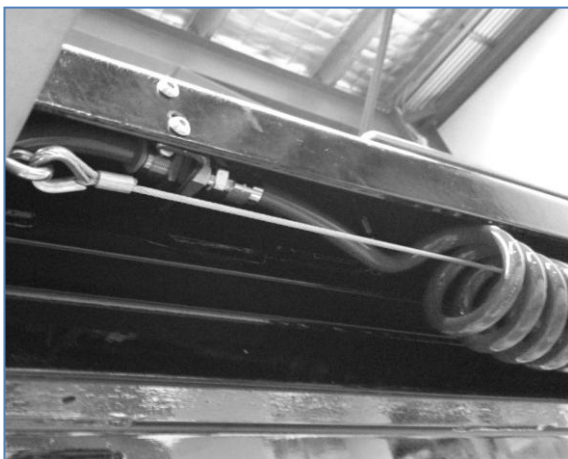
Photos of Coiled Hose (#11) fitted over wire rope assembly between bulkhead and jacking beam.
