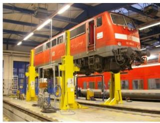
Proportional valve technology synchronously controls all cylinders while a rotary encoder on the nut feeds location data to the electronic system so synchronization of the lifting units is monitored to within a tenth of a millimetre.
