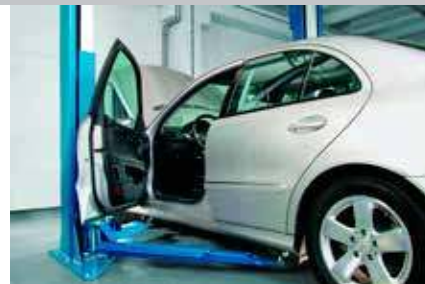
Vehicles's door can be opened completely (2.30 SL DT)
