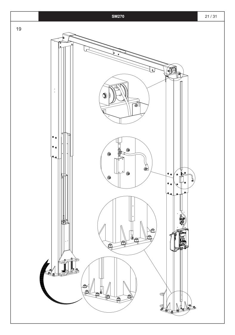
20. Fasten both hydraulic hoses on bottom of cylinder by means of banjo screw connection. **NOTE!** Check at the same time that cylinder is centrered in hole on base plate.
