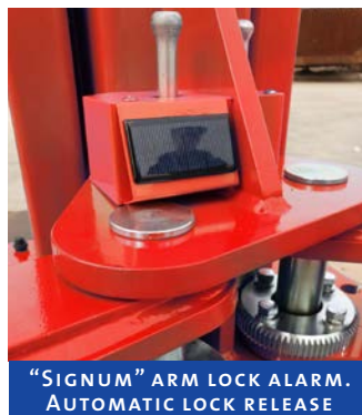
LOW ARM CONSTRUCTION – 95 mm
