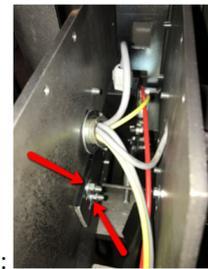
Install with two screw M6x20 (259642), two washer (214620) and two nuts (240308): Adjust the switch to the point where the contact arm is not activated when ratchet is fully engaged in the ratchet rail. Install a switch in each of the other tree columns.
