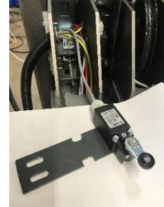
2. Install each the four switches from kit 715317 on the metal bracket (474626): with two washers (214835) on each screw (259609).
