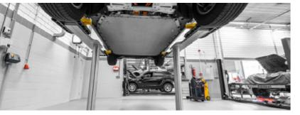
The Masterlift 2.35 Pv 180-240 with piston distance (KA) 1700 can safely lift the most common electric vehicle models currently available.
