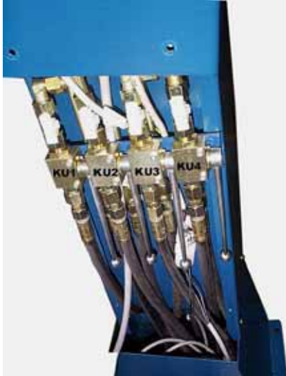
pic. 2: ball valves for the equalization of the lift.
