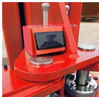
“SIGNUM” ARM LOCK ALARM. AUTOMATIC LOCK RELEASE
