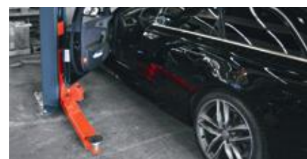
Large door opening angle, door stop protection
