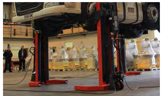
PROGRAMMABLE OPERATION AS GROUPS, PAIRS OR SINGLE COLUMNS
